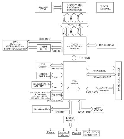
Figure 2.2. Block Diagram
